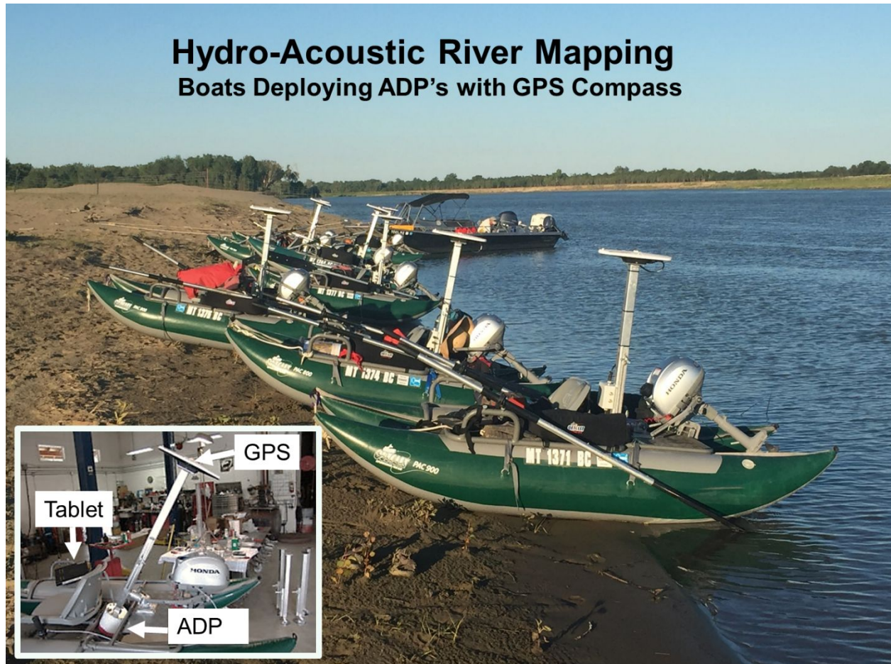
Figure 3. A photograph showing the fleet of small rafts from which the hydroacoustic data were collected. The inset shows configuration of the instruments and field tablet.
